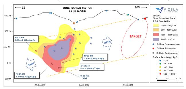
Figure 2: Longitudinal section of the La Luisa Vein.
